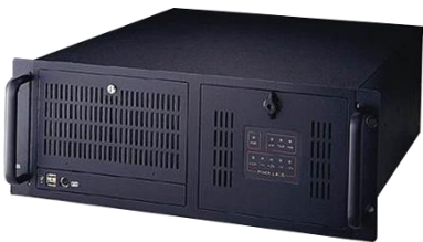
NAVTEX DATA LOGGER
